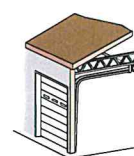
LOW HEADROOM rear mount torsion
