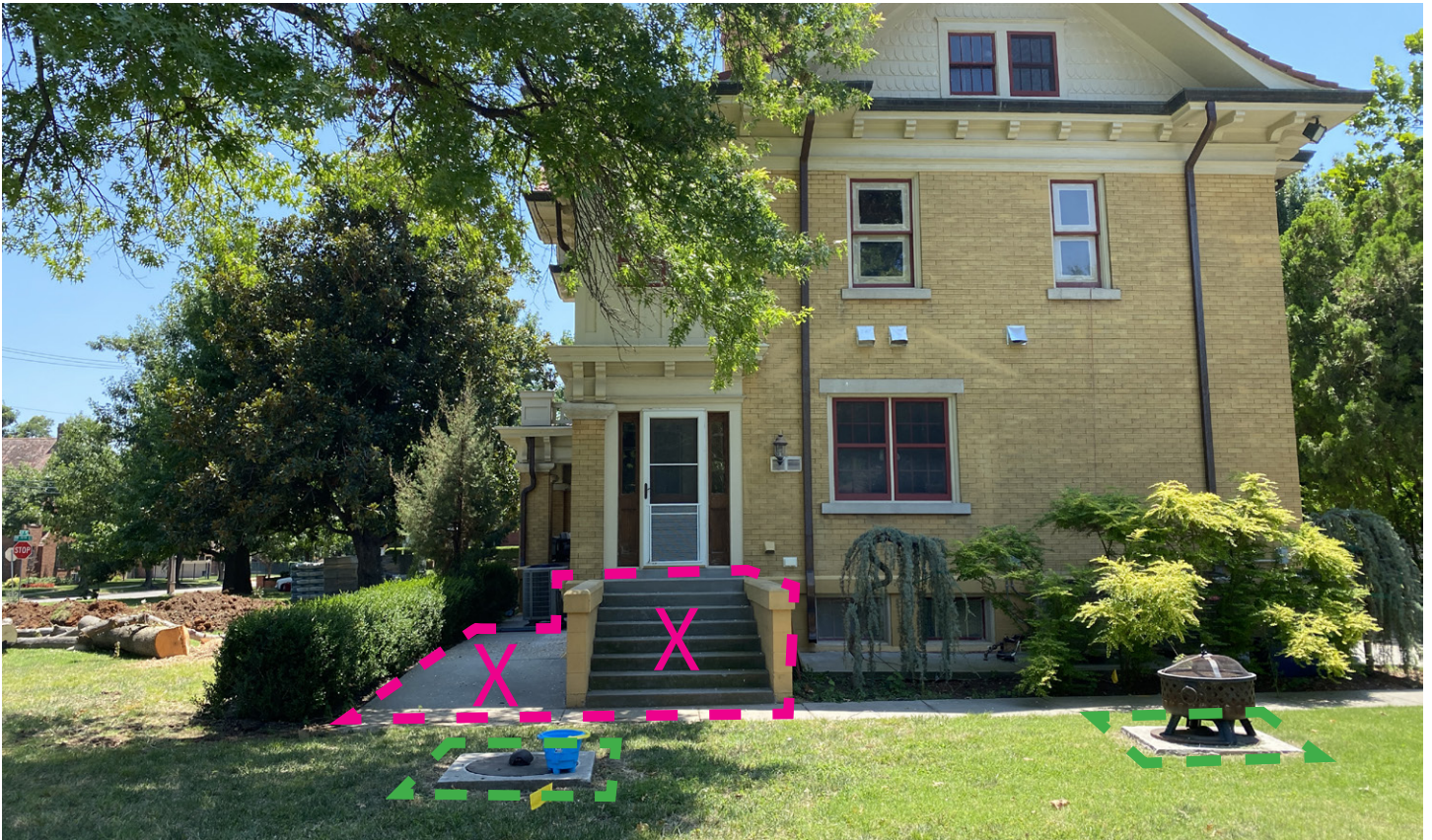
North Elevation Remove north stairs and wingwalls. Keep existing cisterns.
