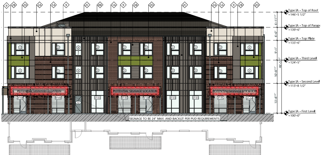
13 Building Type IA - West Elevation Scale: 1/8" = 1'-0"
