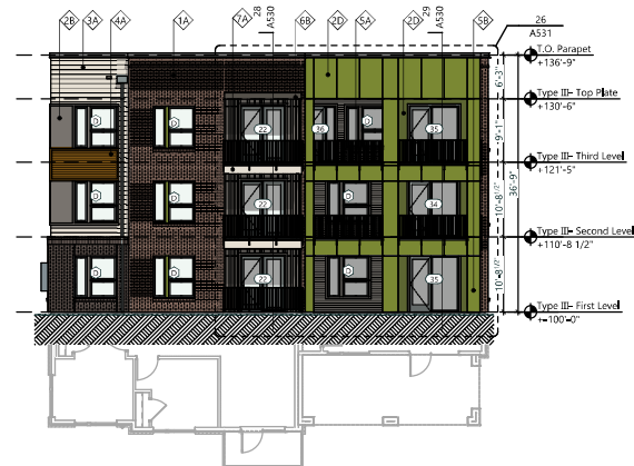
28 Bldg Type III - West Elevation Scale: 1/8" = 1'-0"
