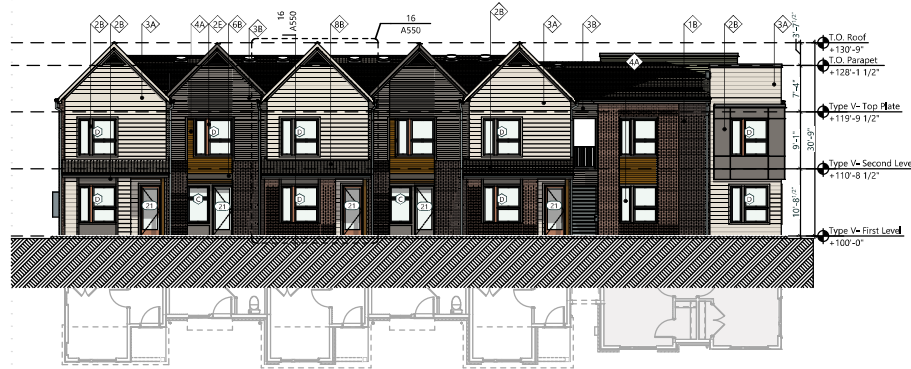
13 Building Type V - South Elevation Scale: 1/8" = 1'-0"
