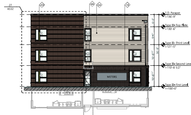
27 Bldg Type III - East Elevation Scale: 1/8" = 1'-0"
