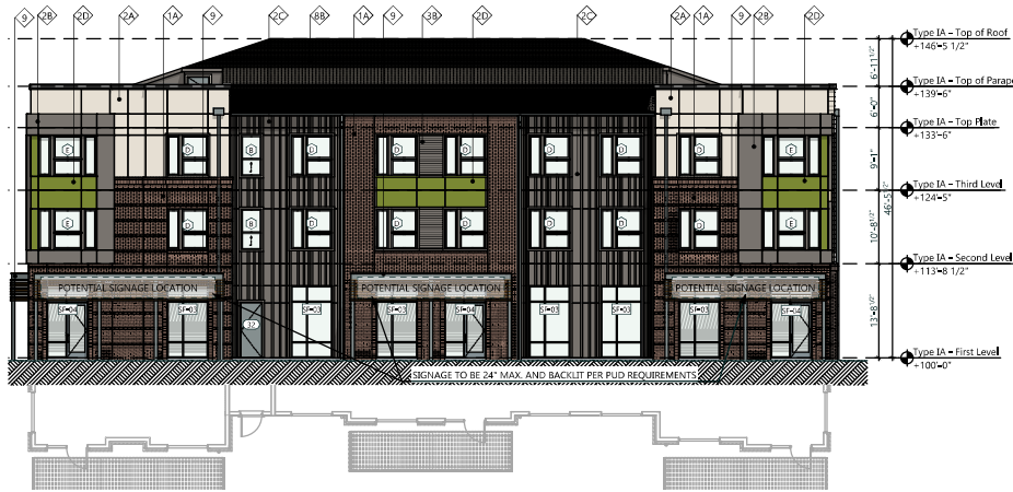
13 Building Type IA - West Elevation Scale: 1/8" = 1'-0"
