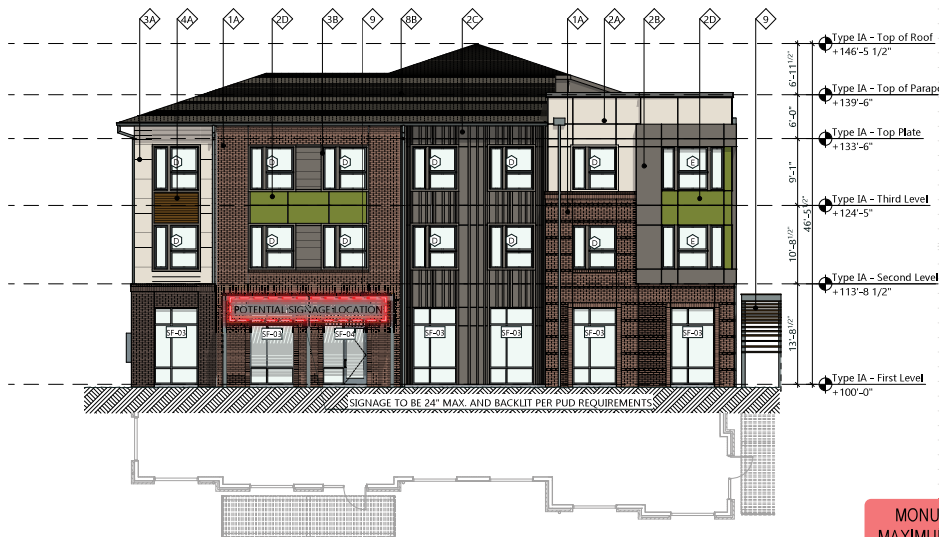
13 Building Type IA - North Elevation Scale: 1/8" = 1'-0"
