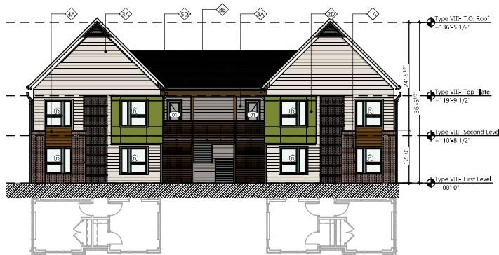
13 Building Type VIII - South Elevation Scale: 1/8" = 1'-0"
