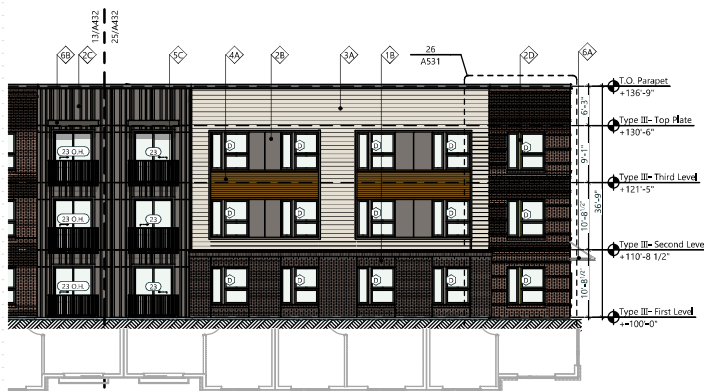
25 Bldg Type III - South Elevation Scale: 1/8" = 1'-0"
