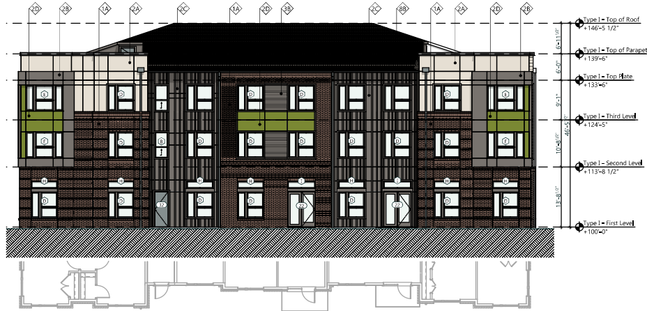
13 Building Type I - West Elevation Scale: 1/8" = 1'-0"
