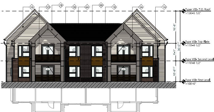
25 Building Type VIII - North Elevation Scale: 1/8" = 1'-0"
