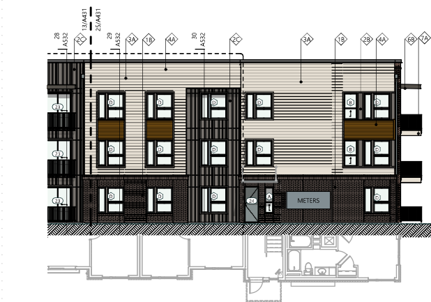
25 Bldg Type III - North Elevation Scale: 1/8" = 1'-0"
