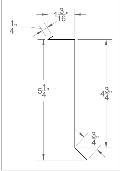
**01** Low Parapet Flashing
