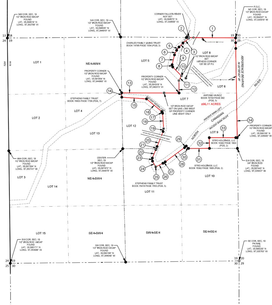
Commencing (P.O.C.) at a found 1/2" Iron Rod by PLS 1200, dated 4-6-2023 for the Northeast corner of said Section 19, being the POINT OF BEGINNING (P.O.B.);
