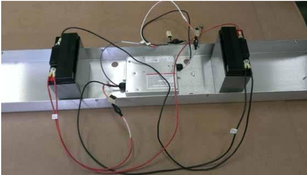
Figure 6. Batteries Wired in Parallel
