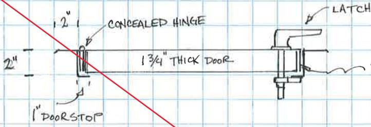
DOOR WILL BE TWO PANELS THAT WILL BE POWDER COATED AND FASTENED TOGETHER WITH POP RIVETS WITH 2" INSULATION SANDWICHED IN BETWEEN
