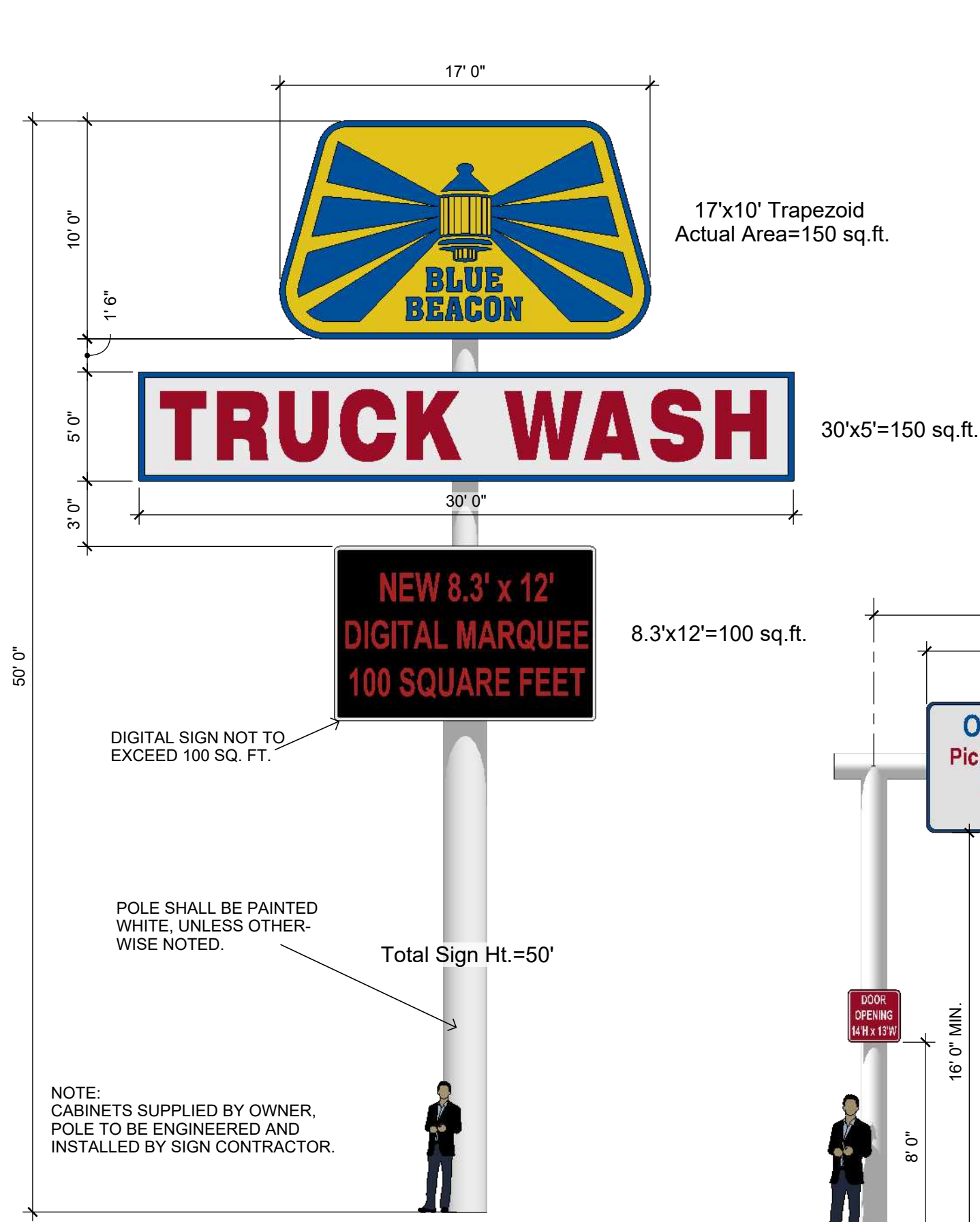
HI-RISE PYLON SIGN (Cabinets Supplied by Owner) GROUND MOUNTED LIGHTING, SEE SITE LIGHTING PLANS
