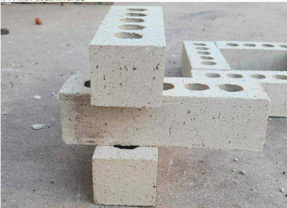
CORNER LAP - PRE-GROUT END CELL WITH PREMIXED
