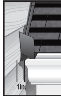
Figure 9 Gutter to Siding
