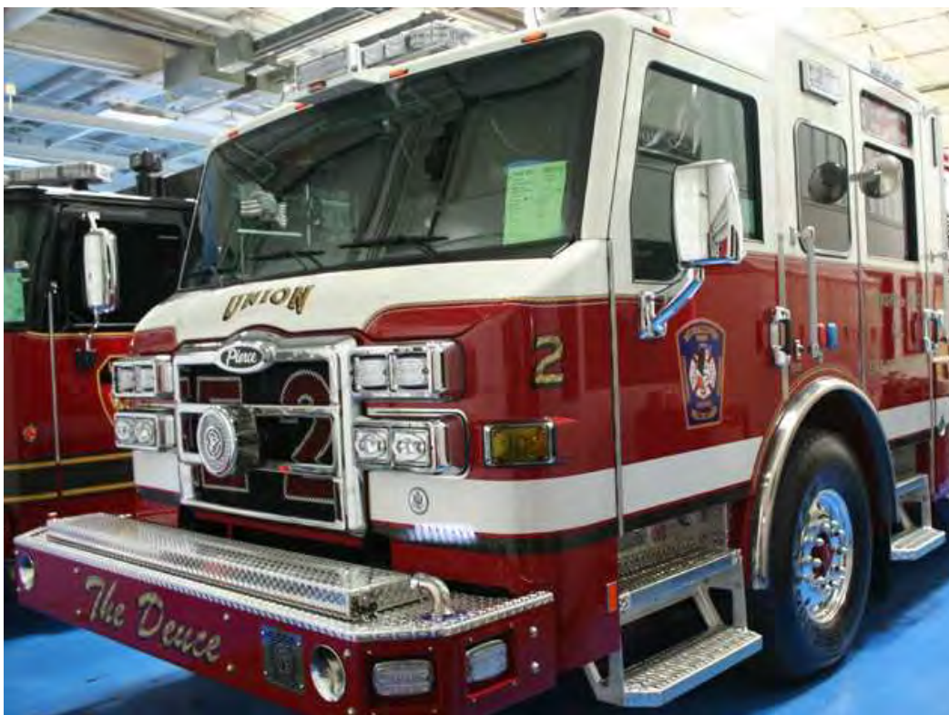
Velocity/Impel – Standard two-tone paint break with high shield
