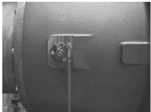
Figure 10. Vane actuator level on suction cover
