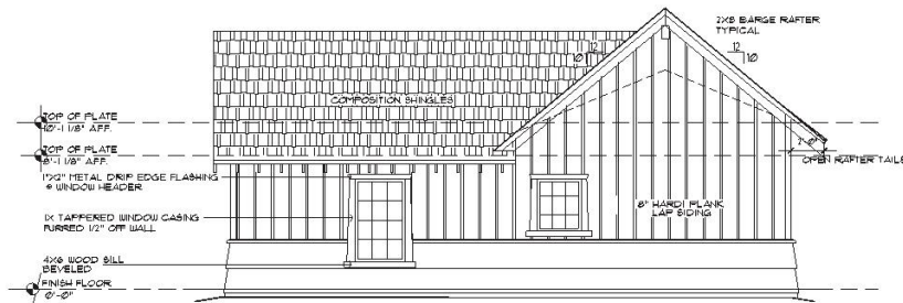
4 SOUTH ELEVATION SCALE: 1/4"=1'-0"
