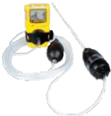
Sampling Hose HOSE1-10/20/65/75 Sampling hose with connectors and 3 particulate filters; available in 10 ft (3m), 20 ft (6.1m), 65 ft (19.8m) and 75ft (22.8m) lengths
