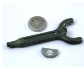
G02-0304-000 PID 10.6eV sensor maintenance kit (includes sensor cap, electrode panel, and cap removal tool) (Used with ToxiRAE Pro family, MultiRAE family and AreaRAE Pro and Plus)
