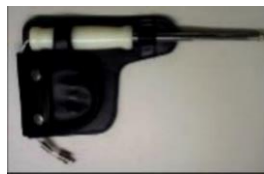
002-3005-000 Collapsible, aluminum remote access probe with insulated handle and 6.5' (2 m) of Teflon tubing. Probe expands to 35"
