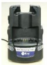
M01-0306-000 Desktop Cradle (AC adapter or PC cable not included): charges the battery, simplifies PC communications, performs PID lamp auto-cleaning
